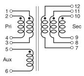
The primary windings and the secondary windings to be connected in parallel on the PC board.
