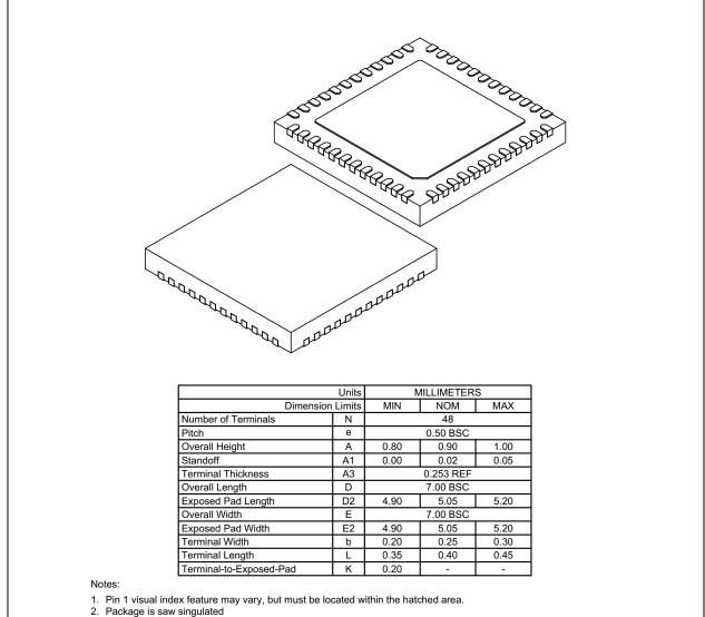
3. Dimensioning and tolerancing per ASME Y14.5M BSC: Basic Dimension. Theoretically exact value shown without tolerances.
