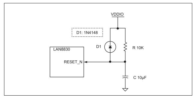
Figure 6-11 illustrates the reset circuit for applications where reset is driven by another device (for example, the CPU or an FPGA). At power-on-reset, R, C, and D1 provide the monotonic rise time to reset the LAN8830 device. The RST\_OUT\_N from the CPU/FPGA provides the warm reset after power-up.
