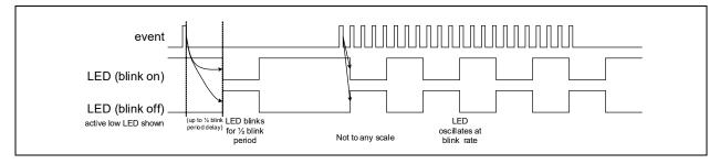
Pulse-stretch guarantees that an LED is asserted and de-asserted for a specific period of time when activity is either present or not present.
