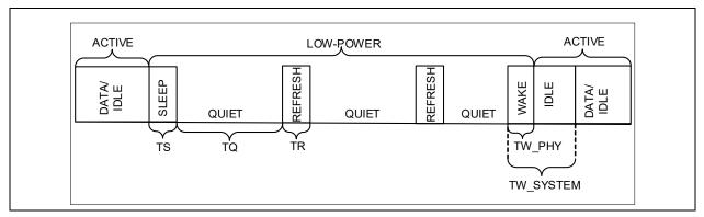
Per the IEEE Standard, the device will wait for one second following link up before sending LPI. This is enabled by default via the lpi\_1sec\_delay bit in the EEE Wait Time Threshold and CRS Block Timer Register.
