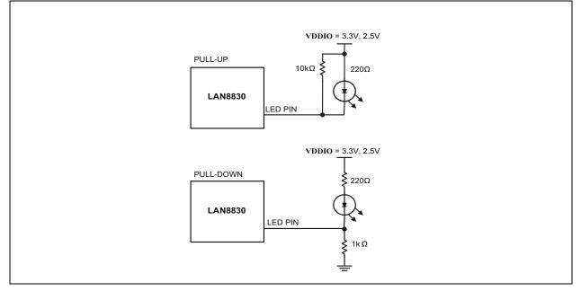
For 1.8V VDDIO, LED indication support requires voltage level shifters between LED[2:1] pins and LED indicator diodes to ensure the multiplexed PHYAD[1:0] strapping pins are latched in high/low correctly. If LED indicator diodes are not implemented, the PHYAD[1:0] strapping pins just need 10 k $\Omega$  pull-up to 1.8V VDDIO for a value of 1, and 1.0 k $\Omega$  pull-down to ground for a value of 0.
