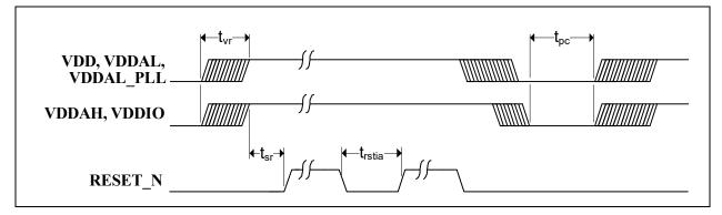
The recommended power-up sequence is to have the transceiver (VDDAH) and digital I/O (VDDIO) voltages power up before the 1.1V core (VDD, VDDAL, VDDAL\_PLL) voltage. If the 1.1V core must power up first, the maximum lead time for the 1.1V core voltage with respect to the transceiver and digital I/O voltages should be 200 µs.
