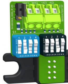
Jumper pins 2-3 120 Ohm
