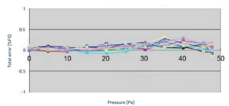
Fig. 1: Typical total accuracy plot of 16 LMI 50 Pa sensors @ 25 °C (typical total accuracy better than 0.5 %FS)
