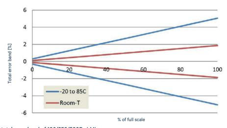
Fig. 2: Maximum total error band of 100/250/500Pa LMI sensors
