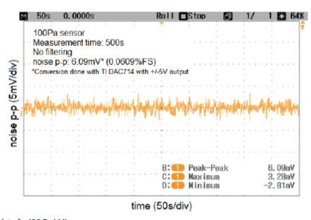
Fig. 3: Typical noise plot of a 100 Pa LMI sensor
