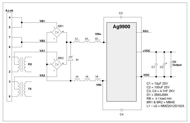
Figure 16: EMC Filtering
