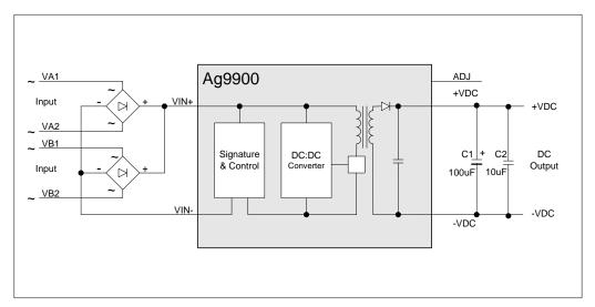
Figure 1: Block Diagram
