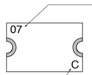
PART IDENTIFICATION: MF-MSHT020KX = 02 MF-MSHT035KX = 03 MF-MSHT050KX = 05 MF-MSHT075KX = 07 MF-MSHT110KX = 11 MF-MSHT125KX = 12 MF-MSHT150KX = 15 MF-MSHT175KX = 17
