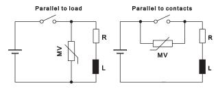
Stabilization of voltages and absorption of line surges
