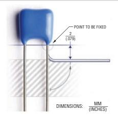
Very often before soldering through-hole components, their leads get bent. It is important not to damage the components during lead bending. Damage most commonly incurred during bending is cracks in epoxy parts, which can lead to increased humidity sensitivity of a component and, consequentially, a shorter lifetime.
