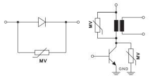
Absorption of piezoelectric alarm shock noise
