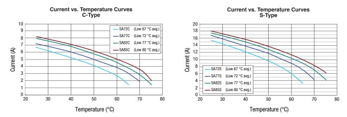
The above curves were derived from placing non-PCB mounted test samples in an oven at 25 °C, 40 °C, 60 °C, and 70 °C, increasing current flow through the sample at a rate of 0.1 A/minute and recording the current value when the sample trips. The current carrying performance is influenced by the PCB design due to copper resistance; users should verify actual device performance in their specific applications.
