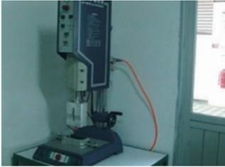
Ultrasonic Welding for Sealing Plastic Case
