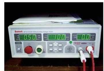
AC/DC Withstanding Voltage Tester
