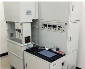
Closed-Loop Wind Tunnel Temperature Chamber
