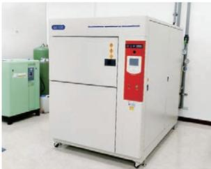
Thermal Shock Testing Chamber
