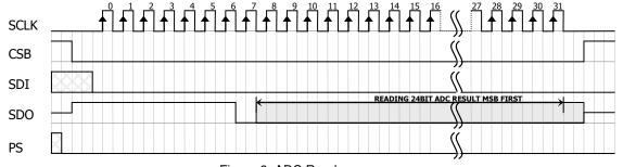
Figure 8: ADC Read sequence
