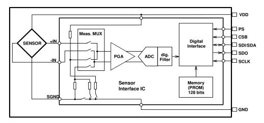
Figure 1: Block diagram of MS5607-02BA
