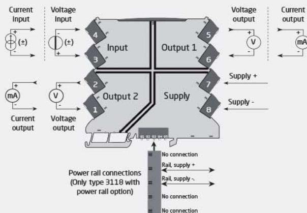
(\* ) Bipolar Input to bipolar output wiring set-up:
