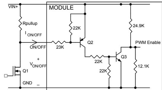
**Figure 42. Circuit configuration for using positive On/Off logic.**
