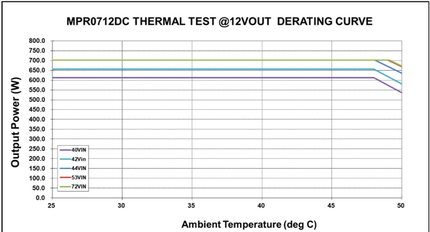
The curves for 40V<sub>IN</sub> and 42V<sub>IN</sub> are only for DCX.
