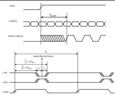
NOTE: LVCK is advanced or delayed with respect to data until errors are observed at the receiver outputs. The advance or delay is then reduced until there are no data errors observed. The magnitude of the advance or delay is RSKM.
